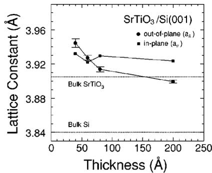
FIG. 2. In-plane and out of plane STO lattice constants for the 40, 60, 80, and 200 Å STO films. The dotted line shows the bulk cubic lattice constant of STO.
