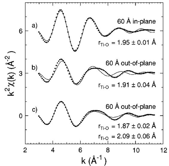
FIG. 4. Fits to the Fourier-filtered, first-shell contributions to the  $k^2$ -weighted Ti  $K$ -edge EXAFS from the 60-Å film using the phase and amplitude functions obtained from the STO powder. The dots are the data points of the back transform, and the solid lines are the fits. (a) In-plane data using one Ti-O distance. (b) Out of plane data using one Ti-O distance. (c) Out of plane data using two Ti-O distances.
