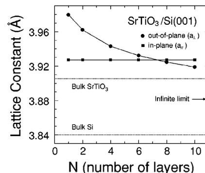
FIG. 5. Calculated out of plane STO lattice constants as a function of supercell size.
