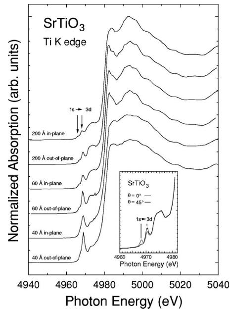
FIG. 3. Ti *K* near-edge x-ray absorption spectra from the thin STO films recorded with the polarization vector in plane and out of plane. The data have been normalized to equal edge jump. The energy positions of the  $1s \rightarrow 3d$  transitions are indicated. The inset shows the pre-edge region of a bulk SrTiO<sub>3</sub> single crystal.
