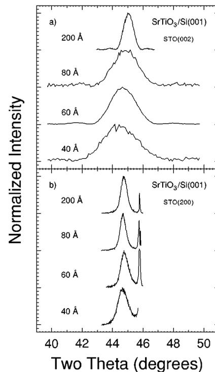
FIG. 1. (a) X-ray diffraction data around the STO(002) Bragg diffraction (out of plane). (b) X-ray diffraction data around the STO(200) Bragg diffraction (in plane).
