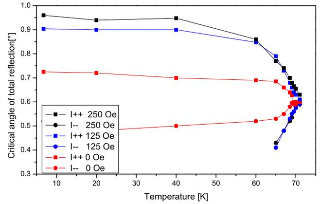
**Figure 5.** Temperature dependence of the critical angle of total reflection of EuO on Si(001) for different temperatures from  $6 \text{ K} \leq T \leq 71 \text{ K}$  and different applied magnetic fields  $B = 0, 125$  and  $250 \text{ Oe}$ . For  $T = T_c$ , the magnetic contribution vanishes. The clear field dependence indicates domain repopulation for increasing external fields in the direction of the applied external field.
