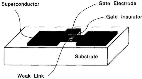
Fig. 6. Sketch of a sample where a superconducting weak link is controlled by an electric field. From [26].
