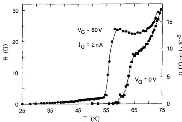
Fig. 7.  $R_{DS}(T)$  curves of an  $\text{YBa}_2\text{Cu}_3\text{O}_{7-\delta}$  film containing weak links for  $I_{DS} = 200$  nA and gate voltages (a)  $V_G = 0$  V, and (b)  $V_G = 80$  V ( $I_G = 2$  nA). From [26].
