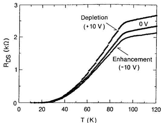
Fig. 2: Temperature dependence of the drain source resistance  $R_{DS}$  of an  $\approx 7$  nm thick YBa<sub>2</sub>Cu<sub>3</sub>O<sub>7- $\delta$</sub>  film for three gate voltages applied: +10 V (solid squares), 0 V (open circles), and -10 V (solid circles). From [13].
