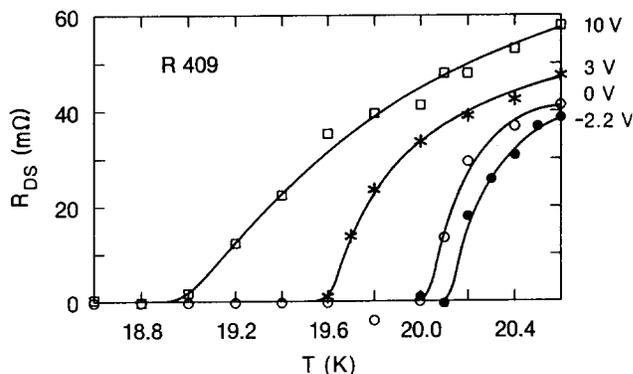
Fig. 3: Temperature dependence (close to  $T_{c0}$ ) of the drain source resistance  $R_{DS}$  of an  $\approx 10$  nm thick YBa<sub>2</sub>Cu<sub>3</sub>O<sub>7- $\delta$</sub>  film for four gate voltages: +10 V (depletion, open squares), +3 V (depletion, stars), 0 V (open circles), and -2.2 V (enhancement, solid circles). For this sample  $R_{DS}(300\text{ K}) \approx 3600\ \Omega$ . From [13].
