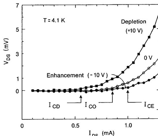
Fig. 4: Current dependence of the drain source voltage  $V_{DS}$  of the YBa<sub>2</sub>Cu<sub>3</sub>O<sub>7- $\delta$</sub>  film shown in Fig. 2 for three applied gate voltages: +10 V (solid squares), 0 V (open circles), and -10 V (solid circles). From [18].
