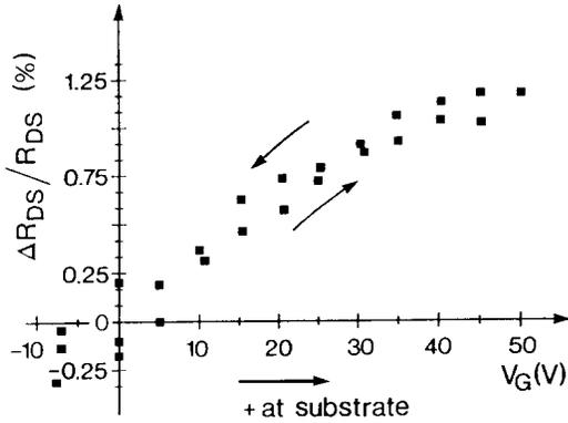
Fig. 5: Change of the drain source resistance  $R_{DS}$  caused by an applied gate voltage  $V_G$  of an  $\approx 10$  nm thick  $\text{YBa}_2\text{Cu}_3\text{O}_{7-\delta}$  film. The change of resistance has been normalized to  $R_{DS}(V_G = 0 \text{ V})$ . The data have been taken at 300 K. From [11].
