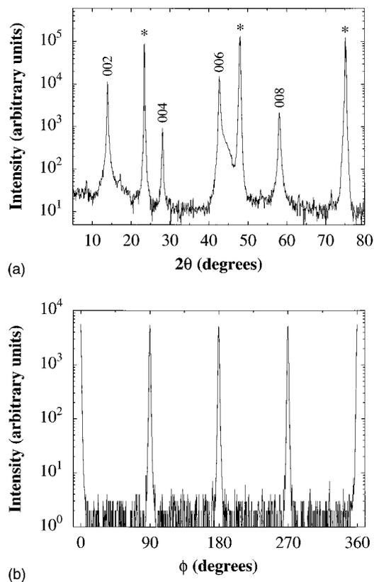
FIG. 1. (a)  $\theta$ - $2\theta$  x-ray diffraction scan of a 2000 Å thick  $c$ -axis oriented  $\text{Sr}_2\text{RuO}_4$  film on a (100)  $\text{LaAlO}_3$  substrate. The substrate peaks are marked (\*). (b) X-ray  $\phi$  scan of the  $\text{Sr}_2\text{RuO}_4$  103 reflection.  $\phi = 0^\circ$  is along the substrate [001] direction.
