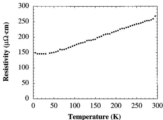
FIG. 3. Resistivity vs temperature for a 2200 Å thick *a*-axis oriented  $\text{Sr}_2\text{RuO}_4$  film on a (100)  $\text{LaSrGaO}_4$  substrate.
