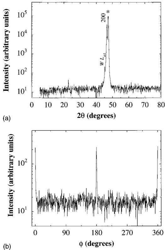
FIG. 2. (a)  $\theta$ - $2\theta$  x-ray scan of a 1700 Å thick *a*-axis oriented  $\text{Sr}_2\text{RuO}_4$  film on a (100)  $\text{LaSrGaO}_4$  substrate. The  $\text{LaSrGaO}_4$  peaks are marked (\*). (b) X-ray  $\phi$  scan of the  $\text{Sr}_2\text{RuO}_4$  305 reflection.  $\phi=0$  is along the substrate [001] direction.
