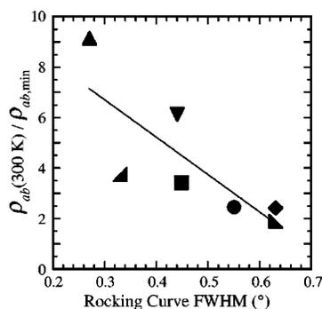
FIG. 4. The resistivity ratios  $[\rho_{ab}(300\text{ K})/\rho_{ab,\min}]$  of the high-purity films shown in Fig. 3, plotted vs the rocking curve FWHM of the 006 peak. High-purity, but crystallographically less-perfect, films exhibit lower resistivity ratios. Symbols correspond to those in Fig. 3.
