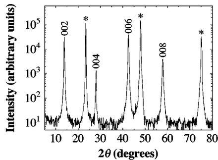
FIG. 1.  $\theta$ - $2\theta$  x-ray diffraction scan of a high-purity PLD-grown  $\text{Sr}_2\text{RuO}_4$  film. This 210-nm-thick film was grown in a background oxygen partial pressure of 3.5  $\mu\text{Torr}$ . The substrate peaks are marked with an asterisk (\*).
