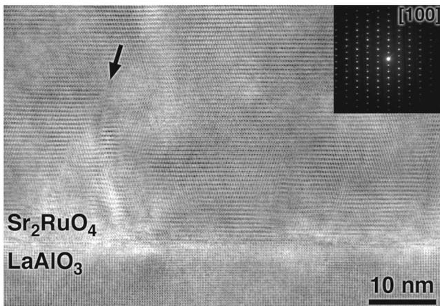
FIG. 2. A HRTEM image of the same high-purity  $c$ -axis  $\text{Sr}_2\text{RuO}_4$  film whose XRD analysis is shown in Fig. 1. The inset shows a diffraction pattern of the  $\text{Sr}_2\text{RuO}_4$  film viewed along the  $[100]$   $\text{Sr}_2\text{RuO}_4$  zone axis.
