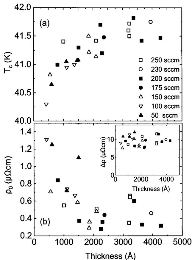
FIG. 4. Thickness dependence of (a)  $T_c$  and (b)  $\rho_0$  of  $\text{MgB}_2$  films made at different  $\text{B}_2\text{H}_6$  gas mixture flow rates. The inset to (b) shows the thickness dependence of  $\Delta\rho = \rho(300\text{ K}) - \rho_0$ .
