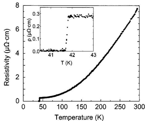
FIG. 3. Resistivity versus temperature for a 2250- $\text{\AA}$ -thick  $\text{MgB}_2$  film deposited at 200 sccm of  $\text{B}_2\text{H}_6$  gas mixture flow rate. The inset shows details at the superconducting transition.
