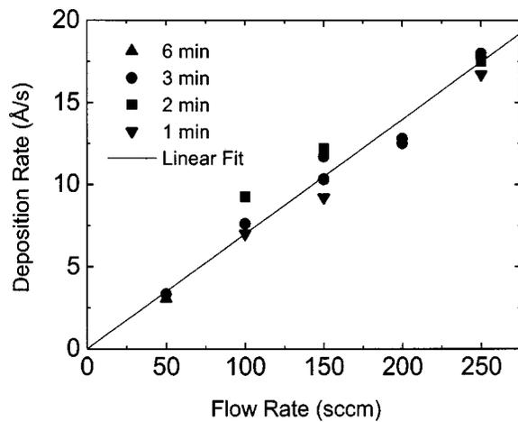
FIG. 1. Deposition rate of  $\text{MgB}_2$  films by HPCVD as a function of the  $\text{B}_2\text{H}_6$  gas mixture flow rate. The data are from films deposited for different lengths of time.
