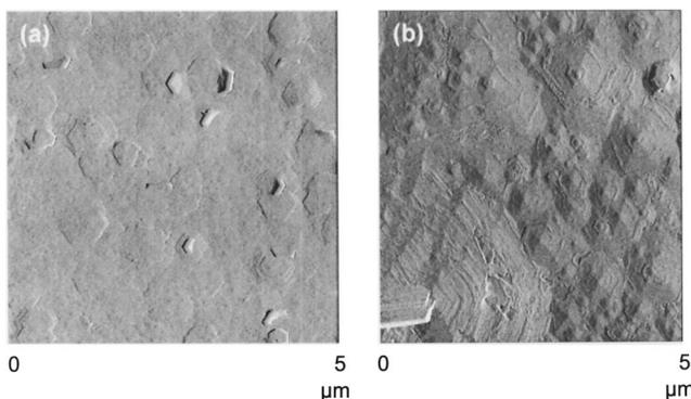
FIG. 2. Atomic force microscopy images of (a) an 840- $\text{\AA}$ -thick  $\text{MgB}_2$  film deposited at 200 sccm of  $\text{B}_2\text{H}_6$  gas mixture flow rate, and (b) a 3400- $\text{\AA}$ -thick  $\text{MgB}_2$  film deposited at 250 sccm of  $\text{B}_2\text{H}_6$  gas mixture flow rate.
