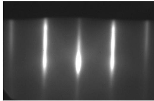
FIG. 2. RHEED image along the  $[110]$  azimuth of EuO after the growth of 660 Å of EuO on a 5-ML buffer layer of SrO on (001) Si on which an interfacial strontium silicide layer was grown.
