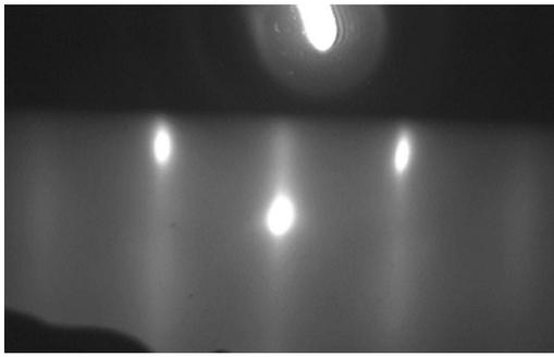
FIG. 1. RHEED image along the  $[110]$  azimuth [of both (Ba,Sr)O and the substrate] of 5 ML of (Ba,Sr)O grown at room temperature on (001) Si using an interfacial europium silicide layer.
