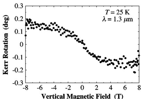
FIG. 5. Polar Kerr response of the same film whose RHEED image is shown in Fig. 2, measured at  $T=25$  K and  $\lambda=1.3 \mu\text{m}$ .
