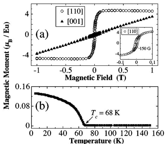
FIG. 4. (a) In-plane  $\mathbf{B}||[110]$  and out-of-plane  $\mathbf{B}||[001]$  hysteresis loops taken at  $T=10$  K. Inset depicts zoomed in  $[110]$  data showing remanence of  $\sim 1.5 \mu_B$  per Eu atom and coercivity of  $\sim 150$  G. (b) Zero-field warming curve with the sample oriented along the  $[110]$  direction reveals a Curie temperature of  $\sim 68$  K.
