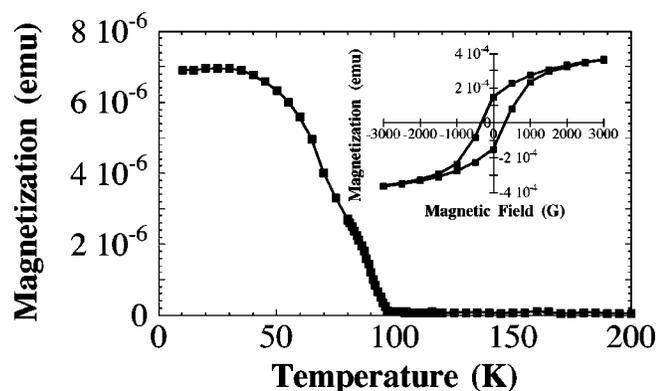
FIG. 4. Magnetization curve of the same BiMnO<sub>3</sub> film as Fig. 1 cooled under no applied magnetic field. The inset shows the ferromagnetic hysteresis loop at  $T=5$  K.
