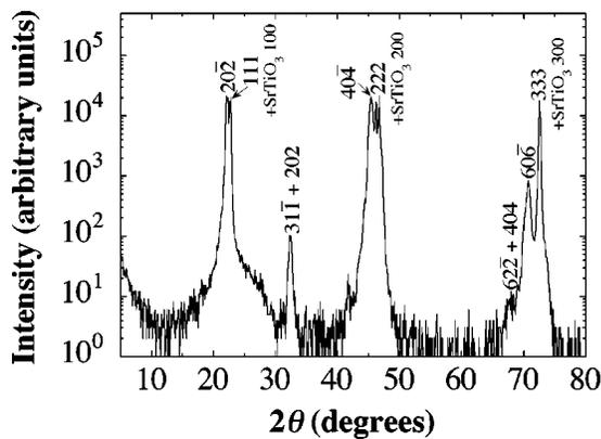
FIG. 1.  $\theta$ - $2\theta$  XRD scan of a  $\text{BiMnO}_3/\text{SrTiO}_3$  film. The full width at half-maximum (FWHM) values for the  $404$  reflection are  $0.44^\circ$  and  $1.1^\circ$  in  $2\theta$  and  $\theta$ , respectively.
