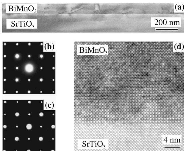
FIG. 3. XTEM images and SAED patterns along the [010] zone axis of the (100) SrTiO<sub>3</sub> substrate of the same BiMnO<sub>3</sub> film as in Fig. 1. (a) Low magnification image, (b) SAED pattern from BiMnO<sub>3</sub> film, (c) SAED pattern from SrTiO<sub>3</sub> substrate, and (d) HRTEM image of the film/substrate interface.
