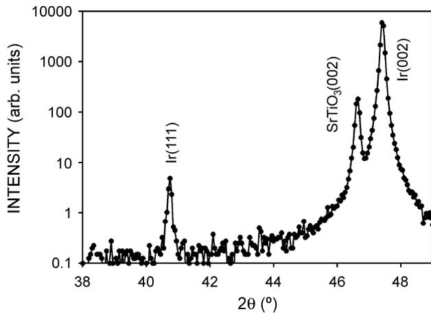
Fig. 2.  $\theta$ - $2\theta$ -scan after deposition of 150 nm Ir on the SrTiO<sub>3</sub>/Si(001) sample.
