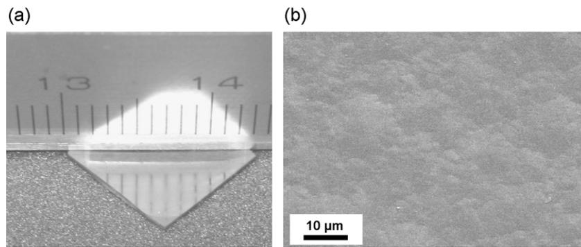
Fig. 6. (a) Optical image and (b) scanning electron micrograph of the thick diamond layer (substrate size 1 cm×1 cm).
