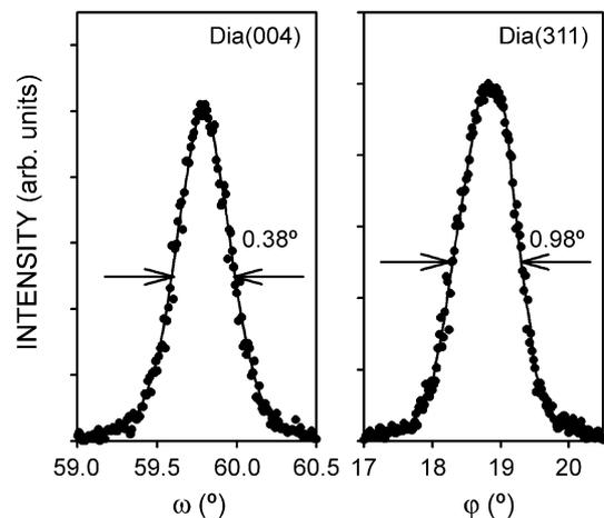
Fig. 5. Diamond (004) rocking curve and diamond (311) azimuthal scan of a 16.5  $\mu$ m thick heteroepitaxial diamond film on Ir/SrTiO<sub>3</sub>/Si(001). The data were fitted by Gaussian curves.
