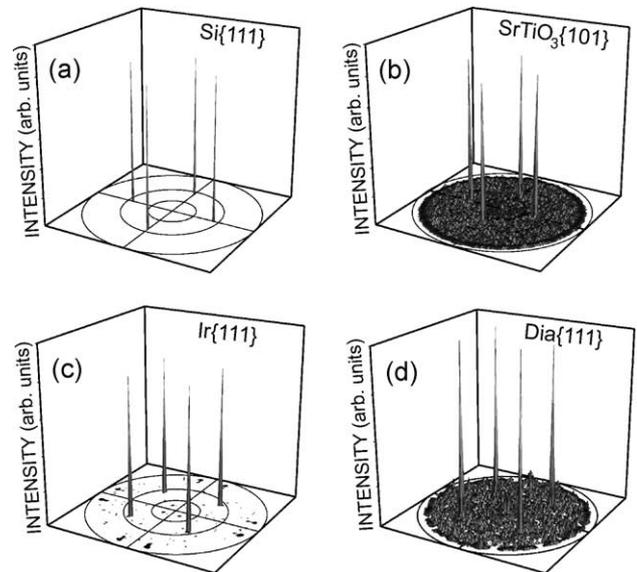
Fig. 4. X-ray pole figures of sample “A” (linear intensity scale).
