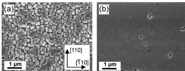
Fig. 3. Scanning electron micrographs of two diamond films grown on Ir/SrTiO<sub>3</sub>/Si(001) substrates. a) Sample “A”: 60 min bias and 60 min growth. b) Sample “B”: 60 min bias and 30 min growth at slightly higher temperature.
