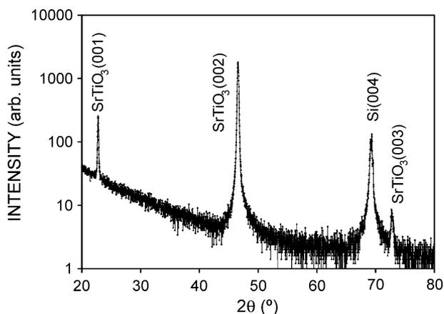
Fig. 1.  $\theta$ - $2\theta$ -scan of a 100-nm thick SrTiO<sub>3</sub> layer on Si(001) grown by MBE.
