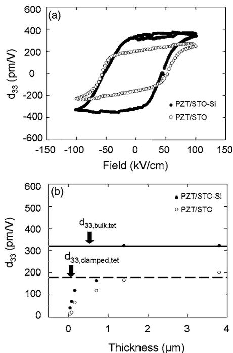
FIG. 4. (a) Typical longitudinal piezoelectric coefficient of 3.8  $\mu\text{m}$  thick PZT films on (001) SrTiO<sub>3</sub> and (001) Si substrates. (b) Thickness dependence of longitudinal piezoelectric coefficient ( $d_{33}$ ) of PZT films on (001) SrTiO<sub>3</sub> and (001) Si substrates.
