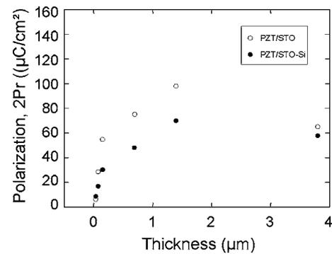
FIG. 3. Thickness-dependent polarization of PZT films on (001) SrTiO<sub>3</sub> and (001) Si substrates.
