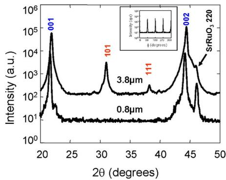
FIG. 1. X-ray diffraction  $\theta$ - $2\theta$  scan of 0.8 and 3.8  $\mu\text{m}$  thick PZT films on (001) Si substrates. The inset shows the azimuthal  $\phi$  scan of PZT 101 reflection, which shows the PZT films on Si growth with cube-on-cube epitaxy.
