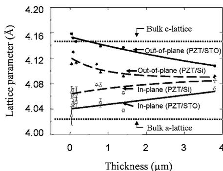
FIG. 2. In-plane and out-of-plane lattice parameters vs film thickness of PZT films on (001) SrTiO<sub>3</sub> and (001) Si substrates.
