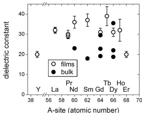
FIG. 3. Dielectric constant  $K$  at 1.7 GHz (right-hand scale) for the series of rare-earth scandates determined by microwave microscopy with the error bars representing the standard deviation of three measurements for each sample. For comparison, bulk dielectric constants (Ref. 3) (measured at 1 MHz) are shown as solid circles (multiple data points indicate the tensor coefficients along the principal axes for single-crystal measurements).
