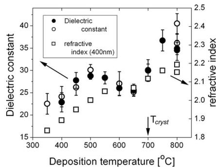
FIG. 2. Dielectric constant  $K$  at 1.7 GHz of  $\text{NdScO}_3$  films deposited at different temperatures (circles, left-hand scale) and their refractive index at 400 nm. Open and solid circles refer to relative permittivities determined from background substrate measurements made before and after the films are measured, respectively, as described in the text. These are placed in the figure to demonstrate the reproducibility of the measurements.
