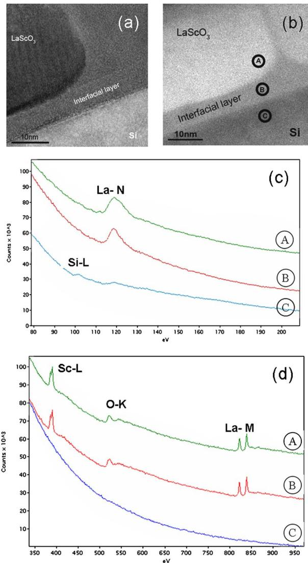
FIG. 2. (Color online) (a) HRTEM image of an ~30 nm LSO/Si (100) stack after 1000 °C, 10 s N<sub>2</sub> RTA, showing an amorphous interfacial layer. (b) High-resolution annular dark field (HRADF) STEM image taken from the area shown in (a). The labeled points designate the location of EELS measurements shown in (c) and (d). EELS spectra were vertically displaced for comparison.
