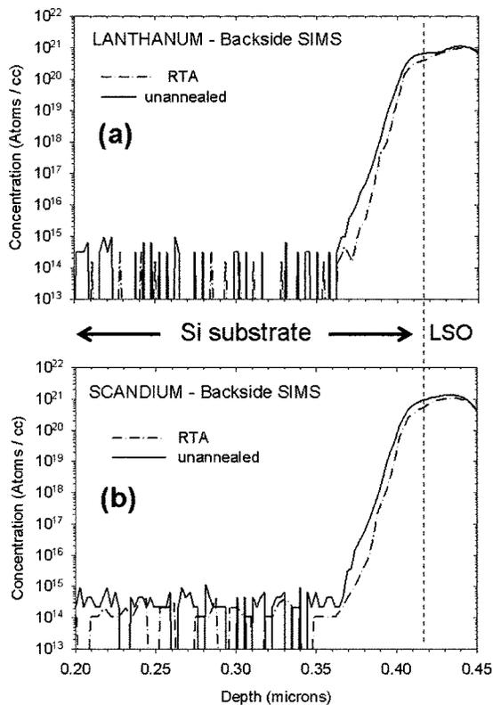
FIG. 1. Back-side SIMS analysis of 100 nm *a*-Si/10 nm LSO/Si (100) stack, before and after 1000 °C, 10 s N<sub>2</sub> RTA. The concentration vs depth profiles of lanthanum are shown in (a) and those of scandium in (b). The silicon substrate was polished to less than 0.5 μm thickness prior to SIMS profiling.
