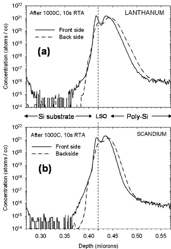
FIG. 3. Front-side SIMS analysis of 100 nm *a*-Si/10 nm LSO/Si (100) stack after the 1000 °C, 10 s N<sub>2</sub> RTA. For comparison of the depth resolution and the ion-beam mixing effects, the corresponding back-side SIMS profiles displayed in Fig. 2 are included.
