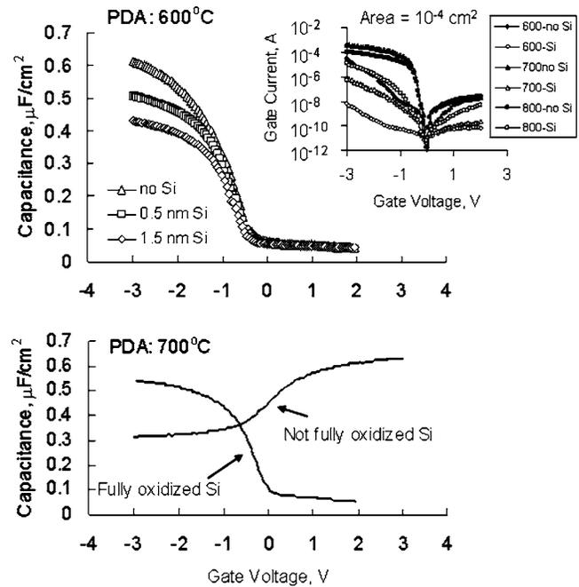
FIG. 1. (a) High frequency (1 MHz) *C-V* characteristics measured on GaAs MOSCAPs with and without *a*-Si IPL after PDA at  $600^\circ\text{C}$ . The inset compares *I-V* characteristics obtained after annealing at various temperatures. (b) *C-V* characteristics on GaAs with fully oxidized and not fully oxidized *a*-Si IPLs after PDA at  $700^\circ\text{C}$ .
