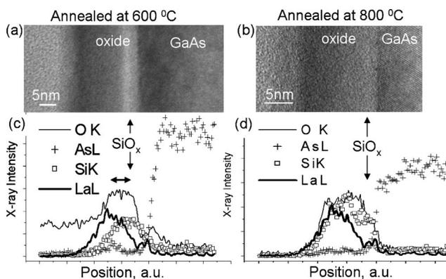
FIG. 3. Cross-sectional TEM/EDX data obtained on GaAs with a fully oxidized 1.5 nm thick  $a$ -Si layer and a 20 nm thick  $\text{LaAlO}_3$  layer after annealing at 600 °C (left) and 800 °C (right).
