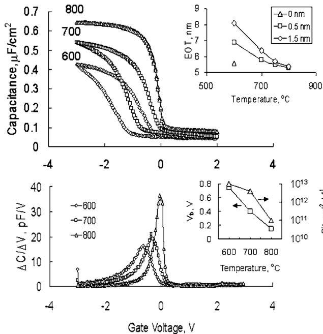
FIG. 2. (a) Effect of annealing on the  $C$ - $V$  characteristics of GaAs MOSCAP with a 1.5 nm thick fully oxidized  $a$ -Si IPL. The inset shows the contribution of the  $a$ -Si to EOT at various temperatures. (b) The improvement of  $C$ - $V$  stretch out with PDA temperature. The inset shows the annealing dependence of  $V_{fb}$  and  $D_{it}$ .
