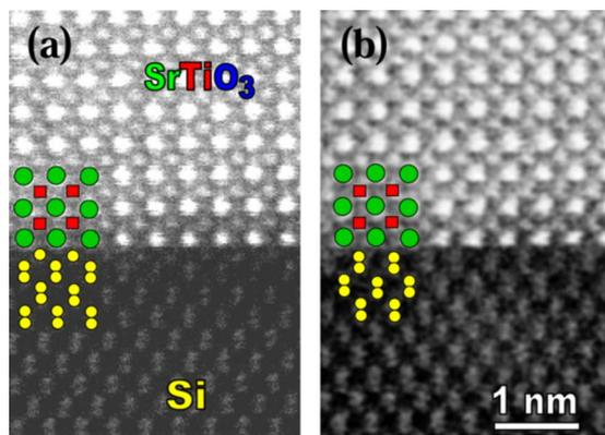
FIG. 1. (Color online) HAADF images of SrTiO<sub>3</sub>/Si interfaces along  $\langle 110 \rangle_{\text{Si}}$ . The atomic arrangement is denoted by colors: green, Sr; red, Ti; and yellow, Si. (a) A plane of Sr(O) facing a silicon plane with a half dumbbell configuration. (b) A plane of Sr(O) facing a silicon plane with a full dumbbell configuration.
