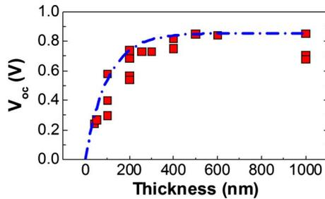
FIG. 3. (Color online)  $V_{OC}$  vs thickness for the ITO/BFO/SRO heterostructures reveals a decrease in  $V_{OC}$  in films less than  $\sim 300$  nm thick.
