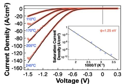
FIG. 2. (Color online) Temperature dependent  $I$ - $V$  measurements on ITO/BFO/SRO heterostructures. Inset, the Schottky modeling fitting of temperature dependent data reveals a Schottky barrier height of  $\sim 1.25$  eV.
