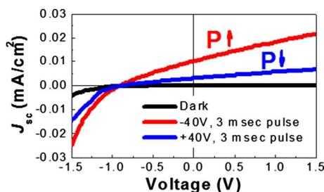
FIG. 4. (Color online) Light (red and blue) and dark (black)  $I$ - $V$  measurements for a ITO/BFO/SRO/STO(111) heterostructure reveals polarization dependent changes in the photovoltaic properties of the device.
