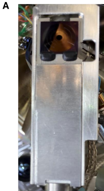
Fig. S3| Collection angle of the DBS detector in DREDI. (A) Photo of the DBS detector in the instrument. (B) Schematic and calculation of the collection angle. The collection angle is between 22.8^\circ to 38.7^\circ .
