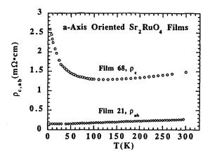
Figure 2. In- and out-of-plane resistivity  $\rho_{ab}$  and  $\rho_c$  vs. temperature T for two *a*-axis oriented films on (100) LaSrGaO<sub>4</sub>. The thicknesses for Films 68 and 21 are 700Å and 2200Å respectively. Both films were rapidly cooled in N<sub>2</sub> after deposition.
