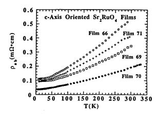
Figure 1. In-plane resistivity  $\rho_{ab}$  vs. T for several *c*axis oriented epitaxial Sr<sub>2</sub>RuO<sub>4</sub> films on (100) LaAlO<sub>3</sub> prepared under various conditions. Film 66 is 3500Å thick and all others are 700Å thick. Film 69 was doped (Sr<sub>1.6</sub>Ba<sub>0.4</sub>RuO<sub>4</sub>) but others were undoped. Films 66 and 69 were cooled rapidly in N<sub>2</sub> after deposition, while films 70 and 71 were cooled slowly in vacuum.
