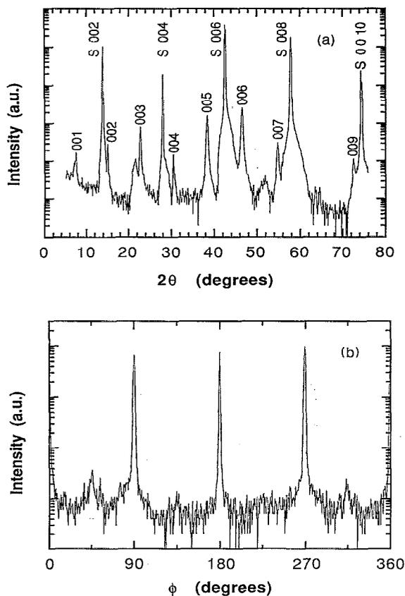
FIG. 3. (a)  $\theta$ - $2\theta$  x-ray diffraction scan aligned to the  $\text{Sr}_2\text{RuO}_4(001)$  substrate plane. The label S denotes substrate peaks. (b)  $\phi$  x-ray diffraction scan of the 103 reflection of  $\text{YBa}_2\text{Cu}_3\text{O}_{7-\delta}$ .  $\phi=0$  is set parallel to the  $\text{Sr}_2\text{RuO}_4[100]$  axis. The  $c$ -axis lattice spacing of  $\text{YBa}_2\text{Cu}_3\text{O}_{7-\delta}$  calculated from the data in (a) is  $c = 11.72 \pm 0.03 \text{ \AA}$ .
