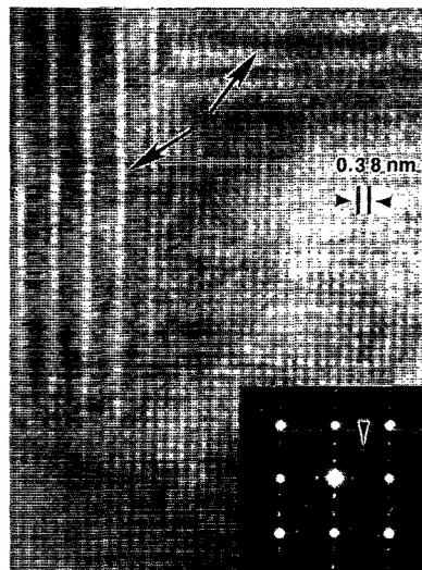
FIG. 4. Plan-view TEM lattice image of an epitaxially grown  $\text{YBa}_2\text{Cu}_3\text{O}_{7-\delta}$  film on  $\text{Sr}_2\text{RuO}_4$ . The  $a$ - $b$ -axis oriented regions are denoted by arrows. The diffraction pattern (inset) clearly shows that aside from the  $\text{YBa}_2\text{Cu}_3\text{O}_{7-\delta}$  reflections, additional spots occur (arrow). They were indexed as  $\text{Y}_2\text{O}_3$ .
