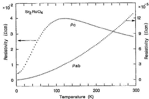
FIG. 1. Resistivity vs temperature of  $\text{Sr}_2\text{RuO}_4$  in the  $a$ - $b$ -plane (indicated by  $\rho_{ab}$ ) and along the  $c$ -axis (indicated by  $\rho_c$ ). See text for discussion of  $\rho_c$ .
