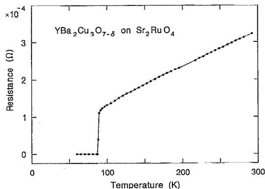
FIG. 2. Resistance vs temperature of a  $\text{YBa}_2\text{Cu}_3\text{O}_{7-\delta}$  film grown on the (001) surface of  $\text{Sr}_2\text{RuO}_4$ .
