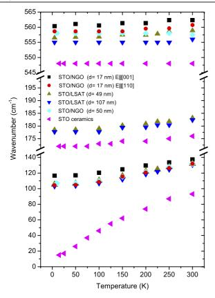
**Figure 10.** Temperature dependences of the polar modes from the polarized IR reflectance spectra of our SrTiO<sub>3</sub>/NdGaO<sub>3</sub> film in comparison with other compressively strained SrTiO<sub>3</sub> films [14, 17] and bulk ceramics [40].
