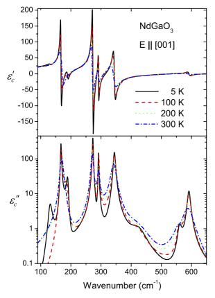
**Figure 3.** Real and imaginary part of the  $\varepsilon_c^*(\omega)$  dielectric function of the (110) NdGaO<sub>3</sub> substrate obtained from fitting its  $E \parallel [001]$  polarized IR reflectivity spectra.
