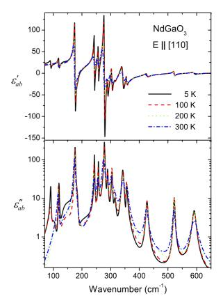
**Figure 4.** Real and imaginary parts of the dielectric function of the (110) NdGaO<sub>3</sub> substrate obtained from fitting the  $E \parallel [110]$  polarized IR spectra. The function represents an arithmetic mean of the  $\varepsilon_a^*(\omega)$  and  $\varepsilon_b^*(\omega)$  functions.
