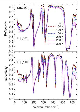
**Figure 2.** Polarized IR reflectivity spectra of a bare (110) NdGaO<sub>3</sub> substrate at selected temperatures.
