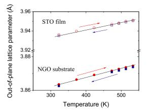
**Figure 1.** Out-of-plane lattice parameters of the (001) SrTiO<sub>3</sub> film and the underlying (110) NdGaO<sub>3</sub> substrate upon which it was grown as a function of temperature on heating (circles) and cooling (squares).
