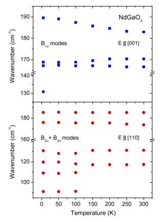
**Figure 5.** Temperature dependence of the low-frequency polar mode frequencies of the (110) NdGaO<sub>3</sub> substrate obtained from fitting the polarized IR reflectivity spectra.  $E \parallel [001]$  polarization yields the  $B_{1u}$ -symmetry modes and  $E \parallel [110]$  polarization yields the  $B_{2u} + B_{3u}$ -symmetry modes.
