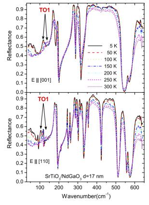
**Figure 6.** Polarized IR reflectance of the 17 nm (001)  $SrTiO_3$  film on the (110)  $NdGaO_3$  substrate.
