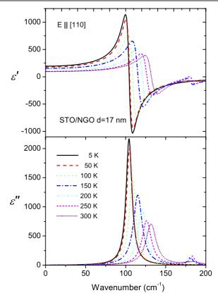
**Figure 8.** Complex dielectric function of the  $SrTiO_3$  film obtained from fitting the  $E \parallel [110]$  polarized IR reflectance of the  $SrTiO_3/NdGaO_3$  system.
