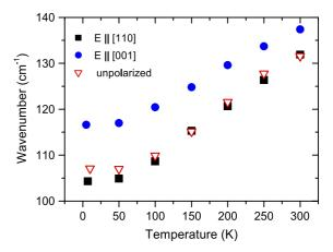
**Figure 9.** Temperature dependences of the in-plane TO1 mode doublet of the 17 nm SrTiO<sub>3</sub> film on the NdGaO<sub>3</sub> substrate from the polarized reflectance spectra in comparison with the TO1 mode from the unpolarized IR reflectance spectra of the 50 nm SrTiO<sub>3</sub> film on the same substrate [14].
