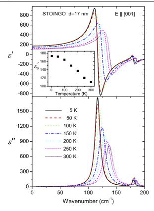
**Figure 7.** Complex dielectric function of the SrTiO<sub>3</sub> film obtained from fitting the  $E \parallel [001]$  polarized IR reflectance of the SrTiO<sub>3</sub>/NdGaO<sub>3</sub> system. Static permittivity obtained from the fit as a function of temperature is shown in the inset.
