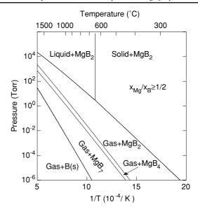
**Figure 2.** The pressure–temperature phase diagram for the Mg:B atomic ratio  $x_{\rm Mg}/x_{\rm B} \geqslant 1/2$ . The region of 'gas + MgB<sub>2</sub>' represents the thermodynamic stability window for the deposition of MgB<sub>2</sub> thin films.
