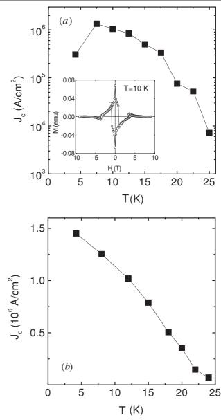
**Figure 4.** The temperature dependence of the zero-field  $J_c$  of a 4000 Å thick MgB<sub>2</sub> film. The inset shows the M–H loop at T = 10 K.
