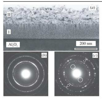
**Figure 5.** (a) Dark-field TEM image showing a cross-sectional view of a MgB<sub>2</sub> thin film with  $T_c = 32$  K. Selected-area electron diffraction patterns from (b) region I and (c) region II.
