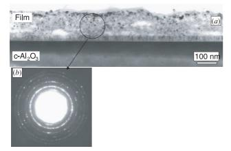
**Figure 7.** (a) Dark-field TEM image showing a cross-sectional view of a second MgB<sub>2</sub> thin film with  $T_{\rm c}=21$  K. (b) Selected-area electron diffraction pattern.
