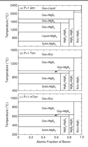
**Figure 1.** The temperature-composition phase diagrams of the Mg–B system under the pressures of (*a*) 1 atm, (*b*) 1 Torr and (*c*) 1 mTorr.
