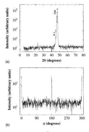
FIG. 2. (a)  $\theta$ – $2\theta$  x-ray scan of a 1700 Å thick a-axis oriented  $Sr_2RuO_4$  film on a (100) LaSrGaO<sub>4</sub> substrate. The LaSrGaO<sub>4</sub> peaks are marked (\*). (b) X-ray  $\phi$  scan of the  $Sr_2RuO_4$  305 reflection.  $\phi$ =0 is along the substrate [001] direction.
