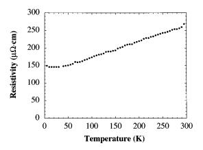
FIG. 3. Resistivity vs temperature for a 2200 Å thick a-axis oriented  $\rm Sr_2RuO_4$  film on a (100) LaSrGaO $_4$  substrate.
