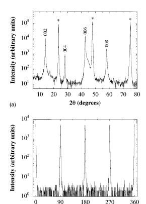
FIG. 1. (a)  $\theta$ – $2\theta$  x-ray diffraction scan of a 2000 Å thick c-axis oriented  $Sr_2RuO_4$  film on a (100) LaAlO<sub>3</sub> substrate. The substrate peaks are marked (\*). (b) X-ray  $\phi$  scan of the  $Sr_2RuO_4$  103 reflection.  $\phi$ =0 is along the substrate [001] direction.
