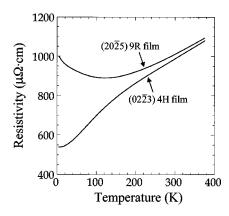
FIG. 3. Temperature dependence of electrical resistivities for both  $(02\overline{2}3)$  4H and  $(20\overline{2}5)$  9R BaRuO<sub>3</sub> thin films grown on (001) SrTiO<sub>3</sub> substrates.
