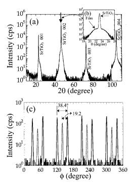
FIG. 1. (a) X-ray normal  $\theta$ -2 $\theta$  diffraction pattern for the BaRuO<sub>3</sub> film on (001) SrTiO<sub>3</sub> substrate at 600 °C; (b) rocking curve measured at 2 $\theta$  = 46.50°. The arrow, "↓", in (a) corresponds to the 02 $\overline{2}3$  4H reflection; (c)  $\phi$  scan patterns of both 30 $\overline{3}0$  and 03 $\overline{3}0$  4H reflections, drawn with solid and dotted lines, respectively.
