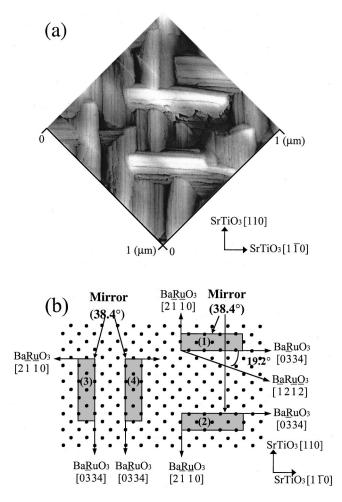
FIG. 2. (a) STM image showing nearly orthogonal domains; (b) schematic drawing of the expected domain structure and epitaxial relation from Fig. 1(c), where the rectangles indicate four  $(02\overline{2}3)$  domains with respect to (001) surface mesh of SrTiO<sub>3</sub> substrate (dots).
