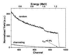
FIG. 2. RBS and channeling measurement of a 1- $\mu$ m-thick BaTiO<sub>3</sub> film on GdScO<sub>3</sub> grown at  $T_{\rm sub}$ =650 °C.
