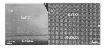
FIG. 3. (a) Cross-sectional TEM of a 1- $\mu$ m-thick BaTiO<sub>3</sub> film grown at  $T_{\rm sub}$ =650 °C on GdScO<sub>3</sub>. (b) Cross-sectional HRTEM of the interface of a BaTiO<sub>3</sub> film grown at  $T_{\rm sub}$ =650 °C on GdScO<sub>3</sub>. The position of the BaTiO<sub>3</sub>/GdScO<sub>3</sub> interface is indicated by the arrows.
