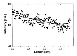
FIG. 5. Scattered intensity from the TE mode for a 1- $\mu$ m-thick BaTiO<sub>3</sub> film grown at  $T_{\rm sub}$ =650 °C on GdScO<sub>3</sub>. The exponential fit gives a loss of 2.2 dB/cm.
