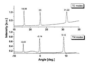
FIG. 4. Bright-line spectra of the TE and TM modes at a wavelength of 632.8 nm in a 1- $\mu$ m-thick BaTiO<sub>3</sub> film grown at  $T_{\rm sub}$ =650 °C on a GdScO<sub>3</sub> substrate
