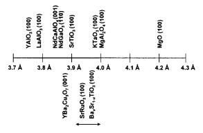
FIG. 1. Approximate lattice constants of the square surface net of several commercially available substrates typically used for the heteroepitaxial growth of oxide thin films. For comparison, the lattice constants of the square surface net of some thin film materials are mentioned below the line. The arrow denotes the lattice parameter range of  $(Ba,Sr)TiO_3$ .
