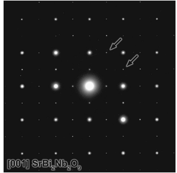
FIG. 4. [001] selected-area diffraction pattern of the \text{SrBi}_2\text{Nb}_2\text{O}_9 film studied by TEM. The superposition of the orthogonal diffraction patterns from the two 90^\circ domain variants leads to an apparent fourfold symmetry. 120 spots unique to the two domain variants are indicated by arrows. Image contrast has been enhanced significantly to show these weak spots; the intensity of major reflections is clipped.
