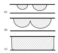
FIG. 4. Schematic depicting (a) nucleation, (b) growth, and (c) combination of dislocation half-loops in epitaxial  $BaTiO_3$  thin films. The inclined portion of the half-loop is called a threading dislocation.
