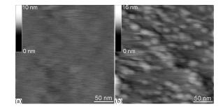
FIG. 5. AFM image of the surface of a 12-nm-thick  $BaTiO_3$  thin film (a) before and (b) after annealing.
