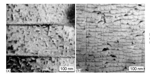
FIG. 1. Planar-view TEM images of the dislocation array in the 8-nm-thick BaTiO<sub>3</sub> film (a) before annealing and (b) after annealing.
