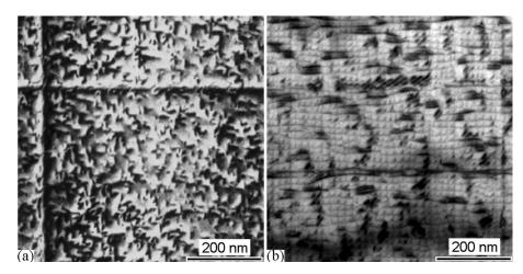
FIG. 2. Planar-view TEM images of the dislocation arrays in the 12-nm-thick BaTiO<sub>3</sub> film (a) before annealing and (b) after annealing.
