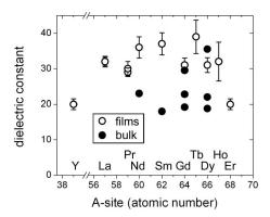
FIG. 3. Dielectric constant *K* at 1.7 GHz (right-hand scale) for the series of rare-earth scandates determined by microwave microscopy with the error bars representing the standard deviation of three measurements for each sample. For comparison, bulk dielectric constants (Ref. 3) (measured at 1 MHz) are shown as solid circles (multiple data points indicate the tensor coefficients along the principal axes for single-crystal measurements).
