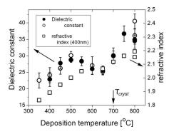
FIG. 2. Dielectric constant K at 1.7 GHz of NdScO<sub>3</sub> films deposited at different temperatures (circles, left-hand scale) and their refractive index at 400 nm. Open and solid circles refer to relative permittivities determined from background substrate measurements made before and after the films are measured, respectively, as described in the text. These are placed in the figure to demonstrate the reproducibility of the measurements.
