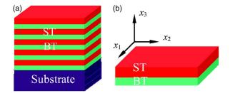
FIG. 1. (Color online) Schematic structures of (a) an epitaxial  $BT_n/ST_m$  superlattice on a substrate and (b) the simulation cell.
