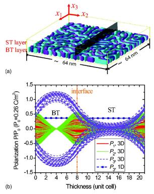
FIG. 3. (Color online) (a) Domain morphology of a  $BT_8/ST_{13}$  superlattice. The two colors in the BT layer indicate domains with up and down polarizations, respectively. (b) Projections of the polarization components  $(P_1, P_2, P_3)$  in the cross section shown in gray in (a) onto a line along  $x_3$  at  $x_1=0$ .
