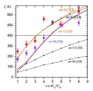
FIG. 2. (Color online) Dependence of  $T_c$  on n and m in commensurate  $BT_n/ST_m$  superlattices on (001) ST substrates. The symbols connected by lines are from the phase-field calculations with multidomain (3D) and single-domain (1D) states, respectively. The scattered solid squares (m = 13) and triangles (m=4) are from UV Raman spectroscopic measurements, and the open squares are from VTXRD measurements (m=4).
