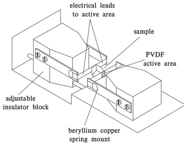
FIG. 1. Schematic diagram of a sample placed between the PVDF transducers with the sample corners maintaining contact with the “active” region.
