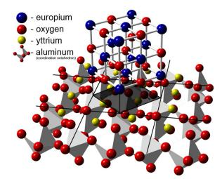
FIG. 1. (Color online) Crystal structure of (001) EuO epitaxially grown on (110) YAlO<sub>3</sub> depicting the  $45^{\circ}$  rotation of the EuO unit cell (above) with respect to the pseudocubic YAlO<sub>3</sub> lattice (below).
