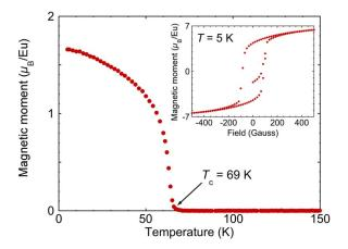
FIG. 5. (Color online) Zero-field temperature dependence of the magnetic moment of a 271±3 Å thick, commensurately strained EuO film grown on (110) YAIO<sub>3</sub>. The onset of ferromagnetism occurs at 69 K. At 5 K, the magnetic hysteresis (inset) shows ferromagnetic behavior with a saturation magnetization of  $6.96\pm0.07~\mu$ B per europium atom, 99.5% of its theoretical maximum.
