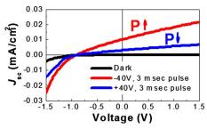
FIG. 4. (Color online) Light (red and blue) and dark (black) *I-V* measurements for a ITO/BFO/SRO/STO(111) heterostructure reveals polarization dependent changes in the photovoltaic properties of the device.
