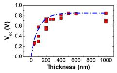
FIG. 3. (Color online)  $V_{\rm OC}$  vs thickness for the ITO/BFO/SRO heterostructures reveals a decrease in  $V_{\rm OC}$  in films less than  $\sim\!300\,$  nm thick.
