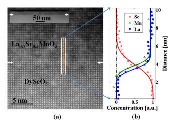
FIG. 2. (Color online) (a) ADF-STEM image of a  $La_{0.7}Sr_{0.3}MnO_3$  film deposited on (110) DyScO<sub>3</sub>, viewed along the [001] zone axis of the substrate ( $\varepsilon_{xx}$ =+1.6%). The inset STEM image shows the film across a 300 nm field of view. (b) Concentration profiles of Sc, Mn, and La across the This a  $La_{0.7}Sr_{0.3}MnO_3/DyScO_3$  interface (arrowed in STEM images). Content is subject to the substrate of the subject to the subject tof
