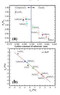
FIG. 3. (Color online) (a) Ratio between the out-of-plane  $(a_{zz})$  and in-plane  $(a_{zz})$  lattice spacing of commensurately  $La_{0.7}Sr_{0.3}MnO_3$  films as a function of the pseudocubic in-plane substrate lattice parameter. (b) The out-of-plane lattice strain  $\varepsilon_{zz}$  as a function of the in-plane lattice strain  $\varepsilon_{xx}$ .
