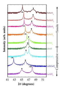
FIG. 1. (Color online)  $\theta$ -2 $\theta$  XRD scans of 22 nm thick La<sub>0.7</sub>Sr<sub>0.3</sub>MnO<sub>3</sub> films grown on different substrates (10 nm thick on NdScO<sub>3</sub>). These substrates impose strains  $\epsilon$  ranging from -2.3% (LaAlO<sub>3</sub>) to +3.2% (NdScO<sub>3</sub>). The arrows ( $\downarrow$ ) indicate the 002 La<sub>0.7</sub>Sr<sub>0.3</sub>MnO<sub>3</sub> film peaks.
