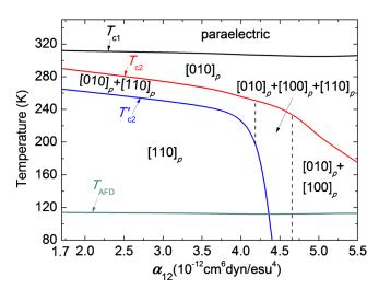
FIG. 3. (Color online) Predicted transition temperatures and polarizations as a function of  $\alpha_{12}$  for SrTiO<sub>3</sub> thin film deposited onto (110) GdScO<sub>3</sub> sub-
