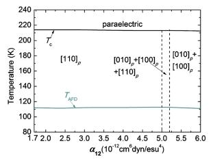
FIG. 1. (Color online) Predicted transition temperatures and polarizations as a function of  $\alpha_{12}$  for SrTiO<sub>3</sub> thin films deposited onto (110) DyScO<sub>3</sub> substrates under a symmetric strain of  $e_{s1} = e_{s2} = 0.94\%$ .
