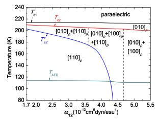
FIG. 2. (Color online) Predicted transition temperatures and polarizations as a function of  $\alpha_{12}$  for SrTiO<sub>3</sub> thin film deposited onto (110) DyScO<sub>3</sub> substrates under asymmetric biaxial strains of  $e_{s1}=1.03\%$  and  $e_{s2}=1.06\%$ .
